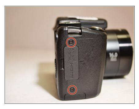
Using the Phillips 00 screwdriver, remove the two 4mm side screws to the left of the LCD screen.
