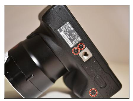
Using the Phillips 00 screwdriver, remove the three 4mm screws from the underside of the camera.
