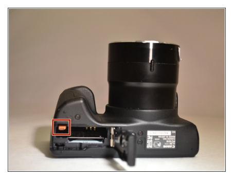
Push the small orange tab forward to release the battery (Battery is ready for removal).
