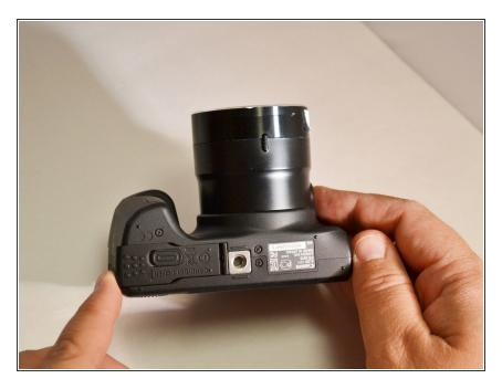
Slide the rounded rectangle tab to the left to release the battery cover.
