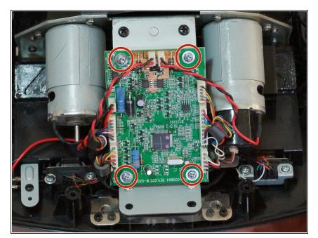
Remove the four 7.3mm silver screws attaching the green PCB board to the motor housing with a Phillips #2 screwdriver.
