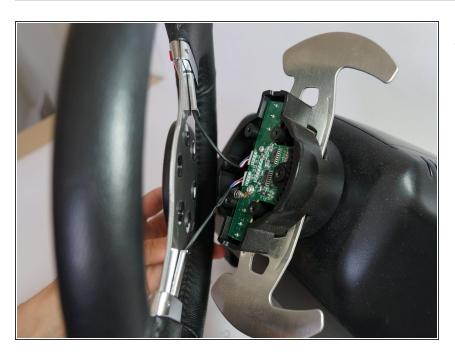
Carefully lift the wheel off of the hub, exposing the 2 shifter paddle wires and PCB board.
