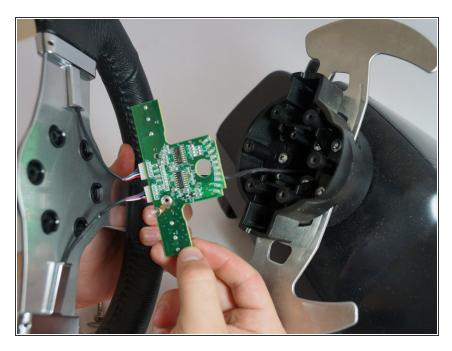
Carefully remove the PCB board from the wheel hub.
