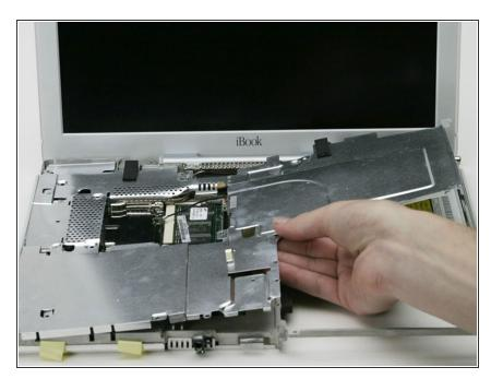
Lift the top shield up from the right side, minding the upper left corner, which may catch on the metal framework.
