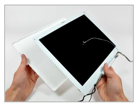
Lift the rear bezel off the display.
