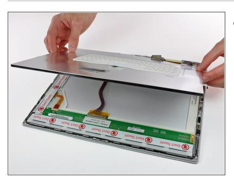
Lift the thin steel LCD cover off the LCD.
