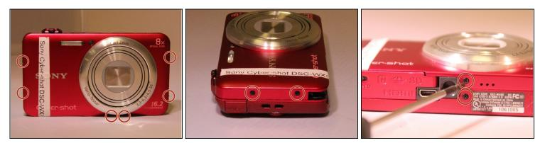
• Remove all six #00 screws holding the outer chassis together with a Phillips #00 screwdriver.
