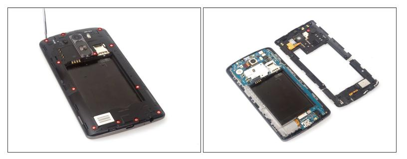
Remove these 12 screws and remove the back frame. Unlike iPhones, these screws are all the same length. The top part of the frame comes with the power button flex while the bottom part of the frame comes with loudspeaker.
