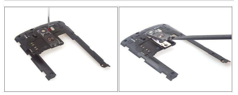
• Remove the black, shorter screw and pry up the power & volume button flex cover.
