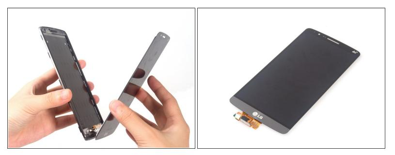
• At last, remove the LCD screen.
