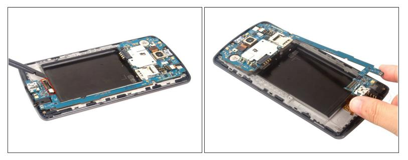
Release the digitizer and LCD connectors. The two cameras are held slightly in the frame.
