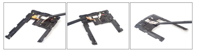
• Carefully loosen the power/volume flex from its adhesive.
