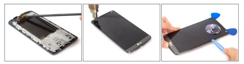
• First, loosen the screen flex from the adhesive on the plate. Then heat the screen edges to melt the adhesive sticker. Next, use the guitar picks and opening tools to cut the sticker.
