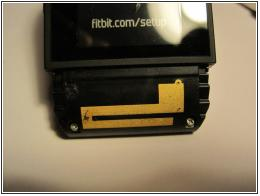
Once you remove the bands scrape away the glue on the top side to expose the GPS antenna
