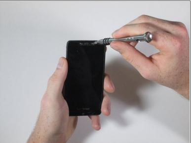
Remove the two 7mm T4 Torx screws at the top of the device.
