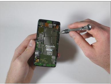
Remove the six 4mm T5 Torx screws located along the outer edge of the motherboard.
