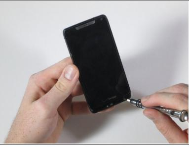
Remove the three T4 Torx screws. There are three at the bottom of the device.
