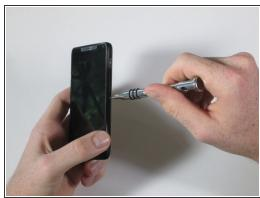
Remove the six 4mm T3 Torx screws. There are 3 on each side of the device.
