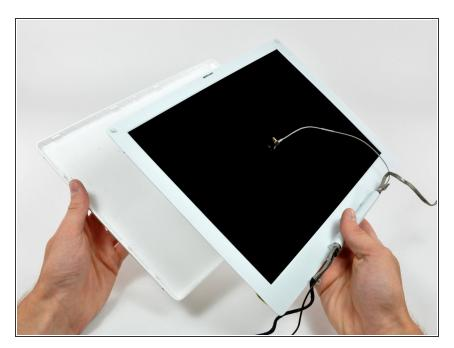
Lift the rear bezel off the display.
