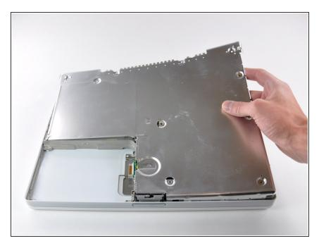
Lift the bottom shield off.
