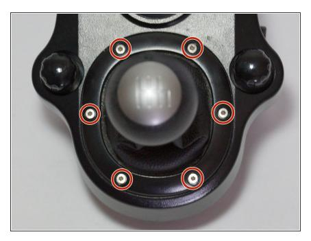
Remove the six 9.0mm allen screws with a 2.5mm hex key.
