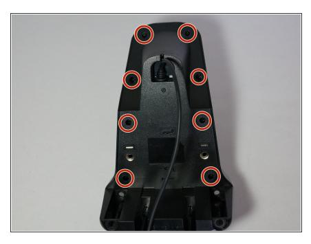
Remove the eight black 11.9mm screws from the bottom housing with a Phillips #1 screwdriver.
