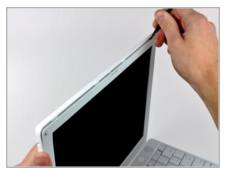
Run your spudger along the top edge of the front display bezel to evenly separate the two bezels.
