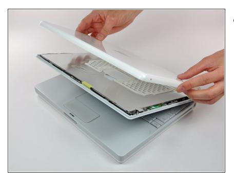
• Lift the rear bezel off the display assembly.
