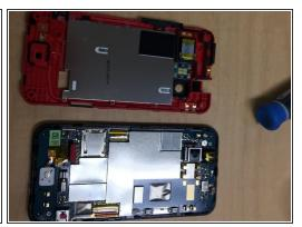
Then remove the three screws. one at the top and the other two at the bottom.
