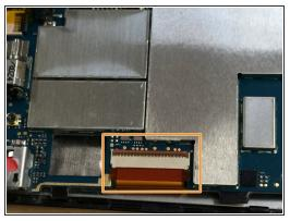
After removing the screw you also have to remove the orange strip by lifting up the top of the container. Then pull the strip out of it.
