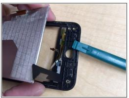
• Remove the top two screws on the pone that will be encased in tape, and then pull the screen out using Blue Opening tool or other.
