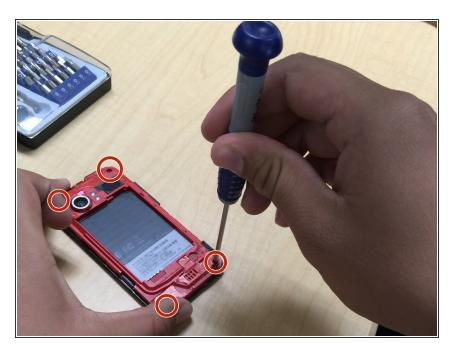
Then remove the four screws located in each corner of the phone.
