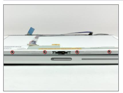
Remove the four small black Phillips screws along the top edge of the display.
