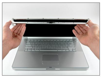
Push the LCD away from the front display bezel near its top edge.
