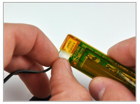
• Disconnect the inverter cable by pulling its connector away from the socket on the inverter board.
