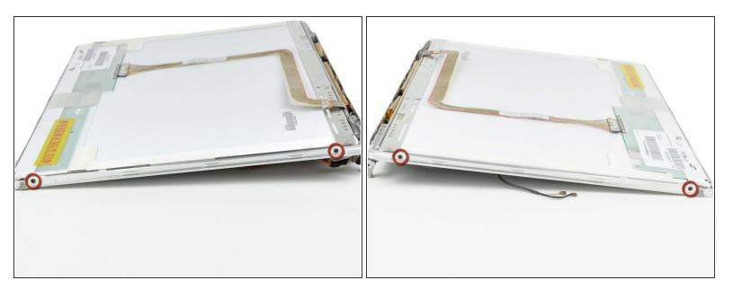
• Remove the two black Phillips screws from both sides of the display (four screws total).
