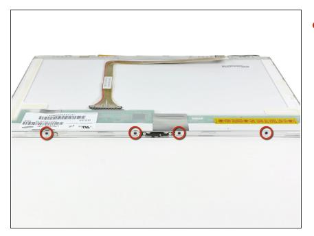
Remove the four black Phillips screws along the top edge of the display.
