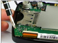
• Remove the three screws holding the motherboard in place.
