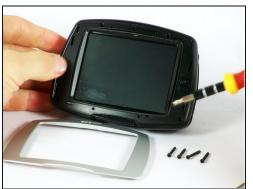
• Use a Phillips #00 screwdriver to remove the four screws around the screen.
