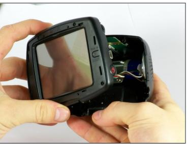
Gently pull from both ends of the casing to separate the front and back panels.
