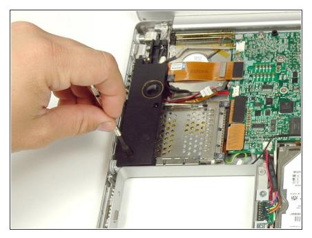
• Remove the 4 mm hex nut securing the left speaker.
