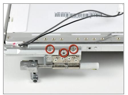
Remove the three 5.7 mm T8 Torx screws securing the right clutch hinge to the front bezel.
