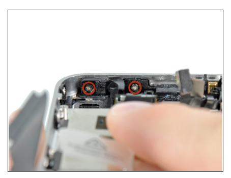
Remove the two 1.5 mm Phillips screws securing the power button bracket to the outer case.
