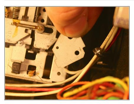
Remove the small steel plate on the right-hand side.
