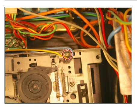
Remove the 5 mm Phillips screw holding the blue and yellow wires in place.
