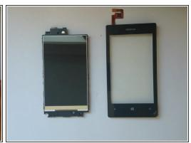
Again use a plastic tool to separate the middle frame and the digitizer frame.
