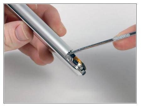
Repeat the same procedure on the other side of the iPhone. Slide the dental pick completely into the square hole. You may need to wiggle the tool and apply a good amount of force to get it to go all the way.
