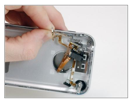
• Lift the headphone jack assembly out of the rear panel.
