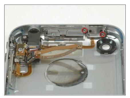
Remove the two Phillips #00 screws securing the on/off switch to the rear panel.
