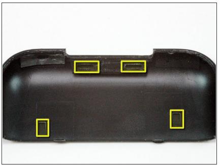
(i) This image shows the two tabs and two catches located on the underside of the antenna cover. The two tabs at the top of the image must be pushed towards the black cover to release them.
