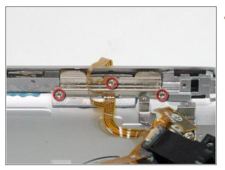
Remove the three Phillips #00 screws securing the volume switch to the rear panel.
