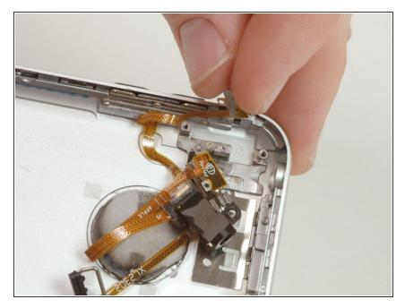
• Grasp the silent/ring switch and lift it up to reveal the screw beneath.
