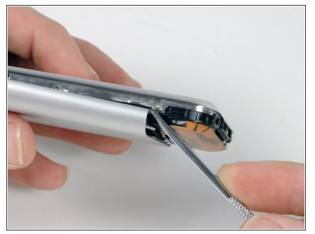
Pry up the rear panel by pulling the dental pick counterclockwise in a quick motion. Apply force perpendicular to the plane of the display assembly. You may be afraid to go fast, but going slowly is more likely to bend the case.
