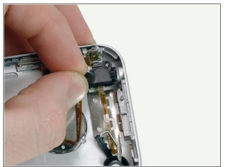
• The headphone jack is slightly recessed into the rear panel. First slide the headphone jack away from its housing and then lift it up slightly (only 1/4 inch or 1/2 centimeter) so that it is no longer in the rear panel.
