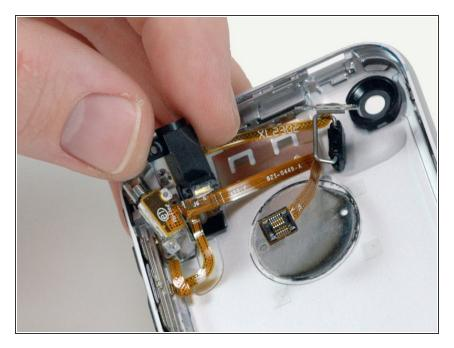
• Grasp the headphone jack at the tip and gently lift up, pulling the vibrator out of the rear panel.
