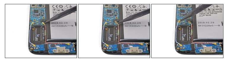
• Use the pointed edge of a spudger to disconnect the Bluetooth and Wi-Fi antenna cable connectors from their sockets on the motherboard.
