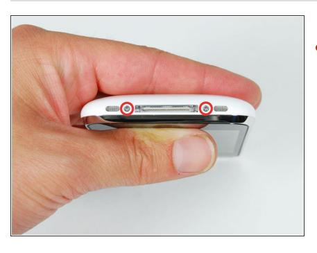
Remove the two 3.7mm Phillips #00 screws from the dock-connector end of the iPhone.
