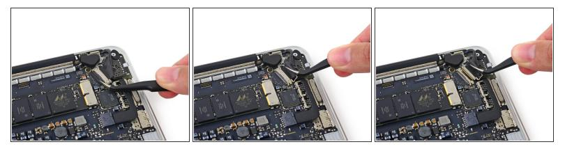
Grab the black plastic tab to flip the display cable connector open and pull it straight out of its socket on the logic board.
