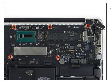
Remove the five 3.5 mm T5 Torx screws securing the logic board to the upper case.
