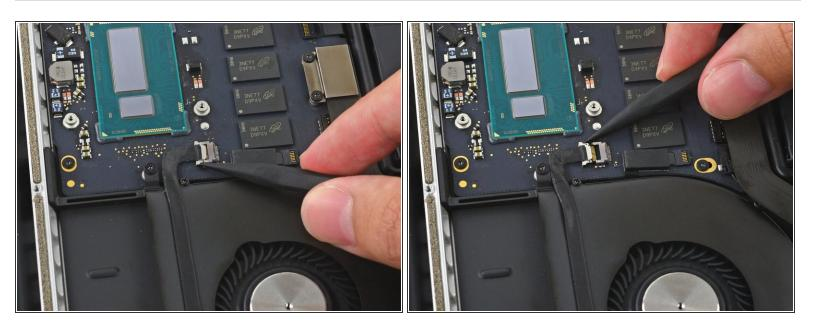
Use the tip of a spudger to push on either side of the the iSight camera cable connector to walk it
