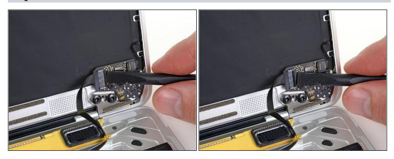
Use a spudger to flip open the retaining flap on the audio jack board cable ZIF connector.
