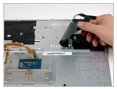
Peel back the black protective sheath on the right side of the upper case. It is not necessary to fully remove this shield. Simply peel it back enough to access the screws beneath.
