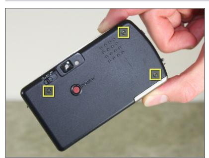
Locate and remove three black 3.80mm screws on the back of the camera with the Phillips #00 screwdriver.
