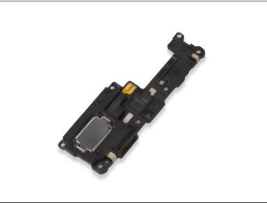
Remove the loudspeaker by prying it up with a spudger.
