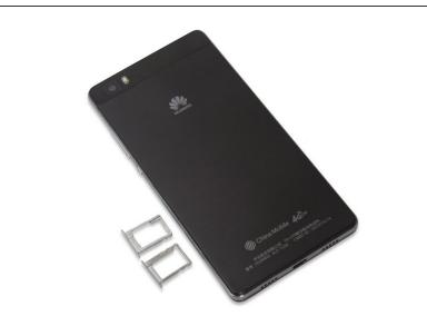
Remove the SIM & SD card trays first.
