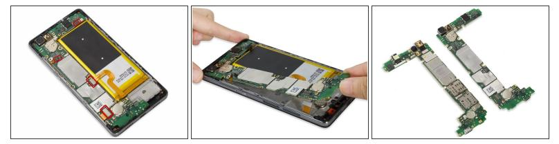
Carefully release all the connectors on the board, and remove the motherboard.
