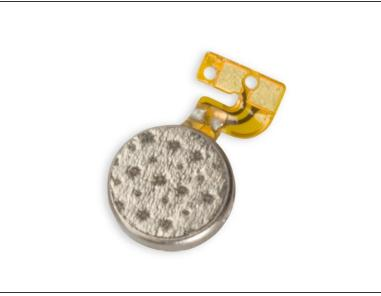
Remove the motor vibrator.
