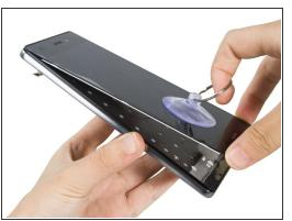
Heat, cut the adhesive sticker and remove the screen carefully.
