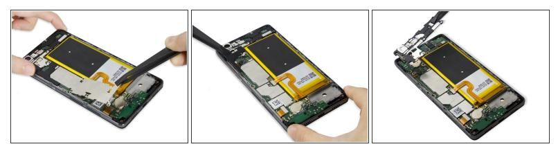
Remove the securing brackets covering the motherboard.
