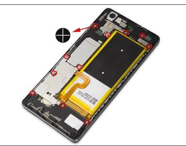
Remove the torx screws on the back.
