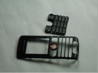
Using the plastic opening tool, press down anywhere on the keypad to separate it from the front case.
