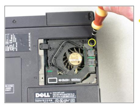
• Remove the single 6mm screw holding the fan in place.
