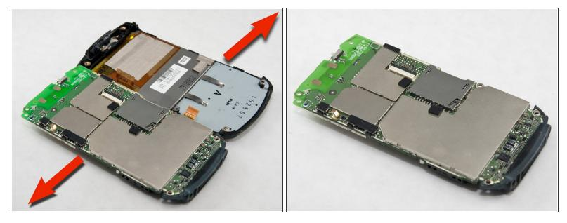
Separate the circuit board from front cover.
