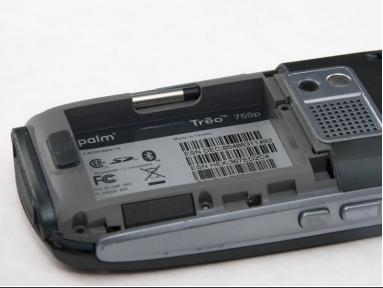
Remove the battery by lifting up on one side.
