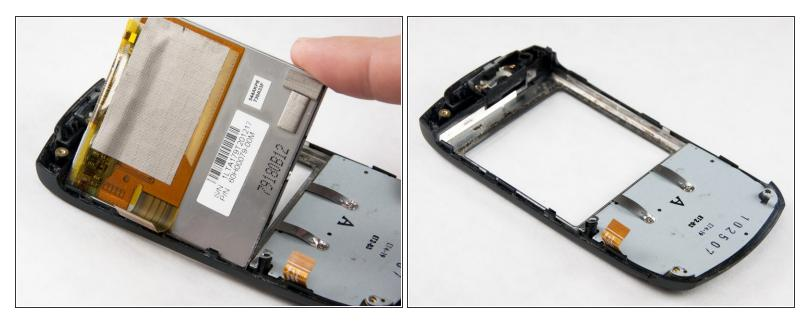
Using your fingers gently lift the display screen panel out of the casing by either grasping it from the back or popping it out of the front.
