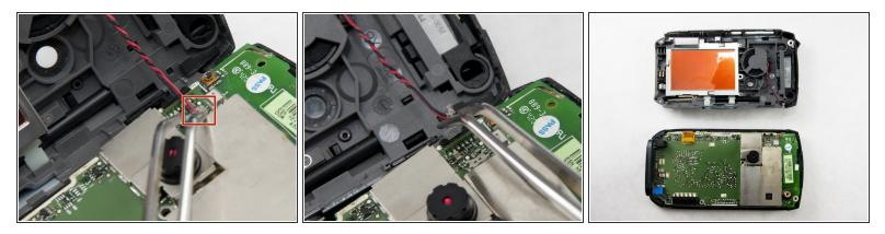
Using tweezers, squeeze the plastic head of the black and red wound wire cable. This will detach
