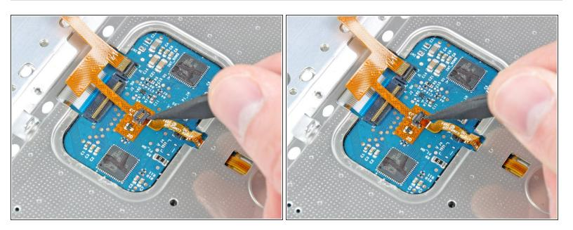
• Use the tip of a spudger to flip up the retaining flap on the mouse button ribbon cable socket.
