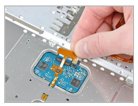
Pull the top upper case ribbon cable connector out of its socket under the trackpad.
