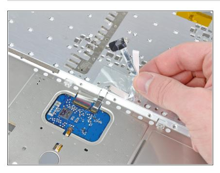
Carefully peel the upper case cable and the piece of clear tape off the bottom of the upper case.
