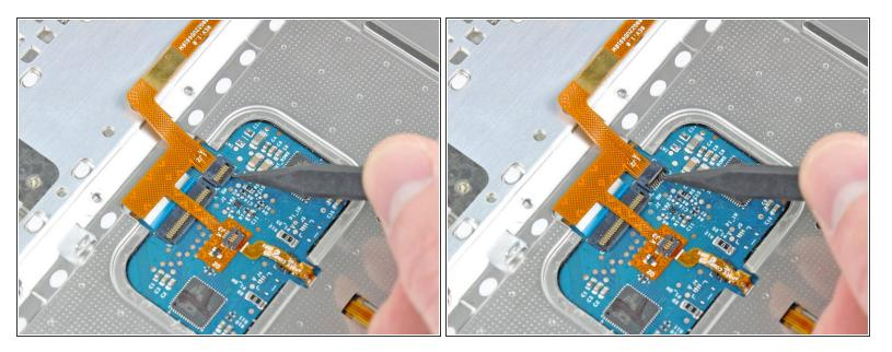
Use the tip of a spudger or your fingernail to flip up the retaining flap on the upper case cable ZIF socket near the keyboard cable.
