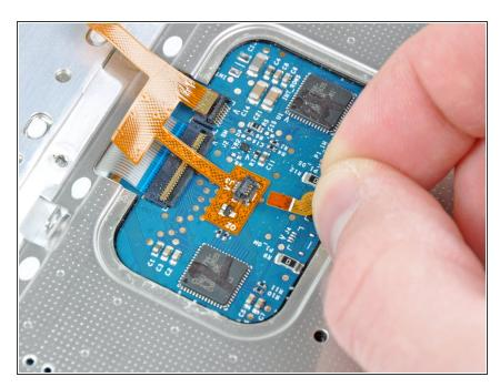
Pull the mouse button ribbon cable out of its socket.
