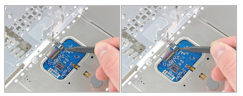
• Use the tip of a spudger to flip up the retaining flap on the upper case cable ZIF socket.
