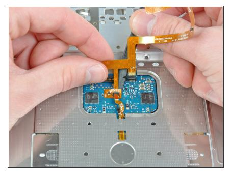
Use the flat end of a spudger to help peel the last portion of the upper case ribbon cable off the adhesive securing it to the underside of the trackpad.
