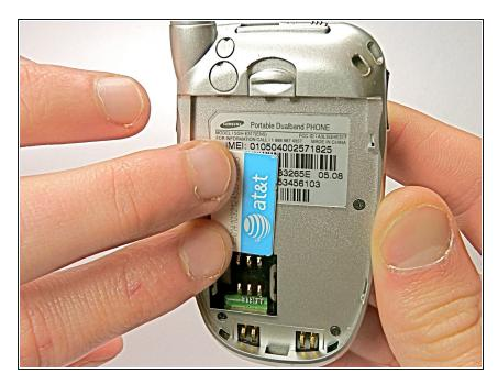
Gently slide the SIM card into the slot, oriented as in the picture.
