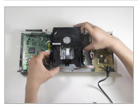
Lift disc drive vertically to remove.
