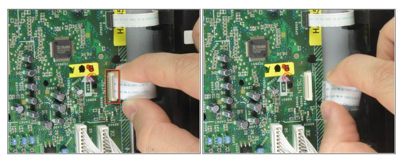
Remove the first of three ribbon cables on left hand side of disc drive by pulling vertically.
