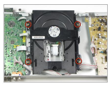
Remove the four screws holding the disc drive in place using a #0 Phillips screwdriver.
