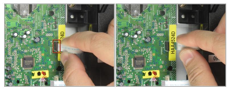
Remove the second of three ribbon cables on left hand side of disc drive by pulling vertically.
