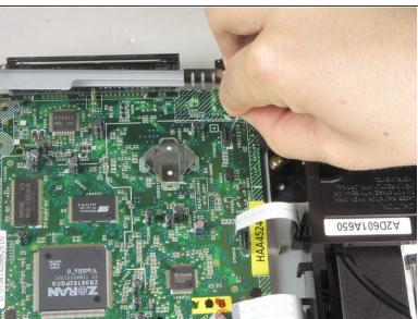
Remove the third of three ribbon cables on left hand side of disc drive by pulling vertically.
