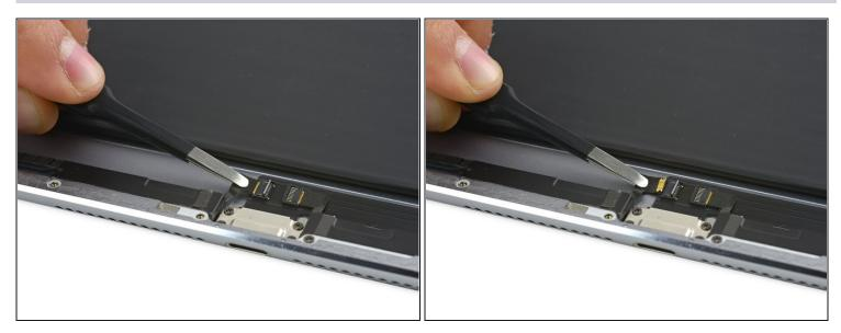
• Slide the speaker cable out of its ZIF connector.
