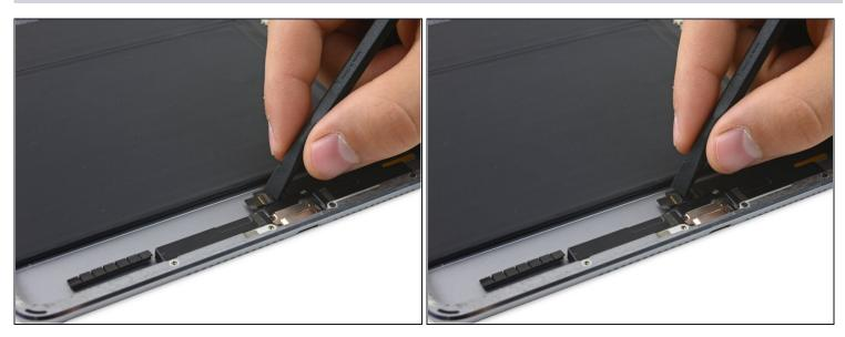
• Use the flat end of a spudger to flip up the retaining flap on the left speaker ZIF connector.
