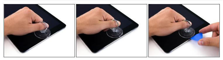
• Firmly pull up on the suction cup to create a small gap between the front panel and the rear case.
