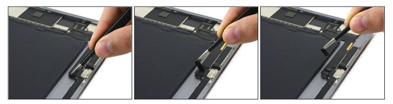
• Remove the tape covering the speaker ZIF connectors.
