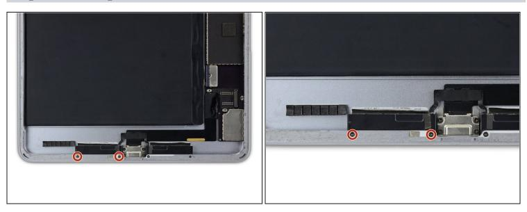
• Remove the two 1.5 mm Phillips #00 screws to the left of the Lightning port.
