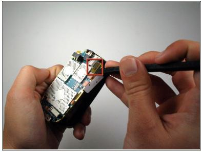
• Use the spudger to lift off the yellow clip near the top right corner of the motherboard.
