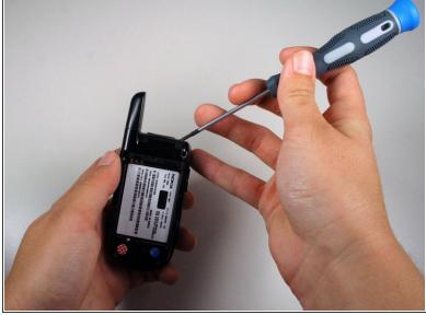
Use a Phillips #00 screwdriver or your fingers to remove the rubber tabs at top back of the phone.
