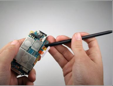
Use the spudger to pull off the top orange chip attached to the white tab.
