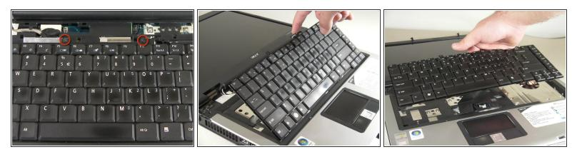
• Under the panel, remove the two screws that connect the keyboard to the laptop.
