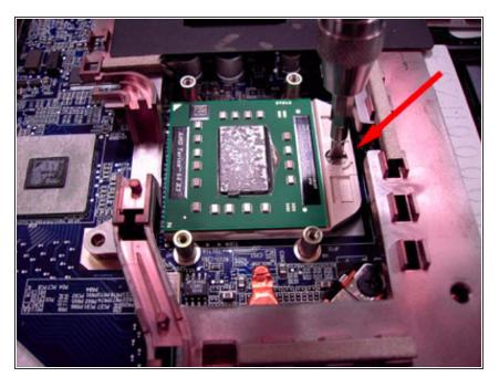
Loosen the screw to the CPU by rotating counter clockwise. The use of a flat head screwdriver will be needed.
