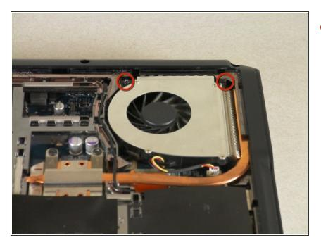
Remove the two screws attached to the fan.
