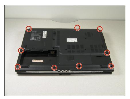
• Remove the nine screws from the back edges of the laptop.
