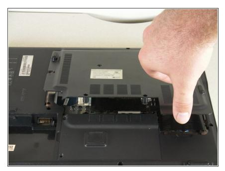
• Lift and remove the panel.
