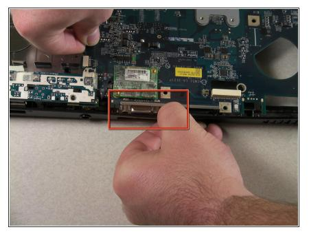
Push out the back of the casing by the VGA connector to remove the motherboard.
