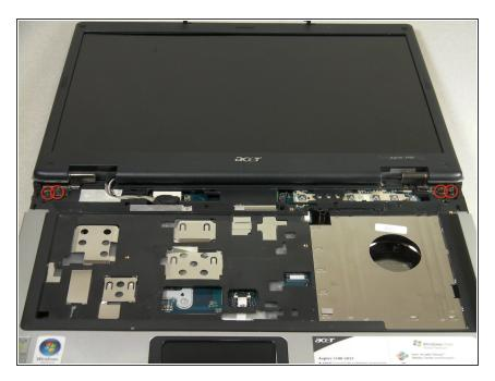
• Remove the two screws from each corner beneath the LCD screen.
