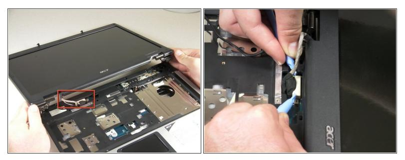
Detach the white rectangle located on the motherboard at the end of the wire connected to the LCD screen.
