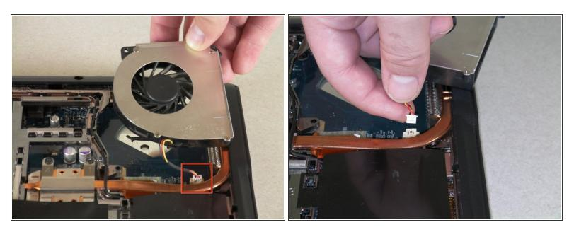
Lift the fan and detach the cable that connects the fan to the motherboard.
