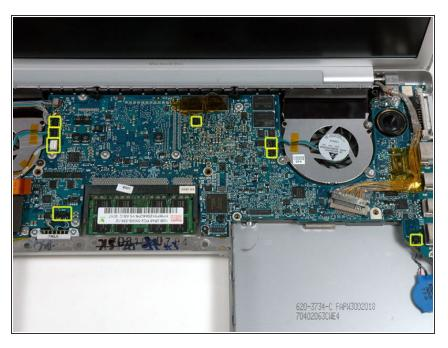
Disconnect the eight indicated connectors by placing a spudger beneath each cable and lifting up.
