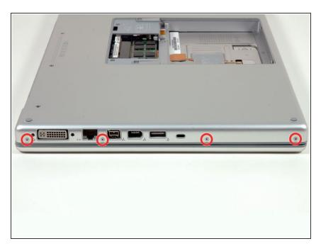
Remove the four 3.2 mm Phillips screws on the port side of the computer.
