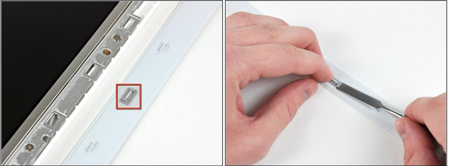
ⓘ Sometimes when removing the front display bezel, the retaining clips that should remain captive in the LCD brackets come out with the front display bezel. Follow this and the next step to transfer the clips back to the LCD bracket.
