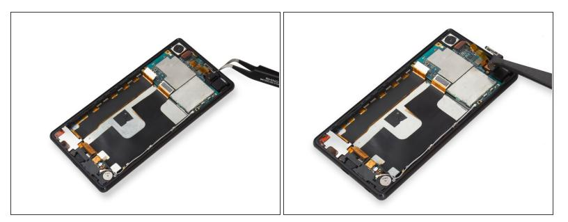
• Remove that small securing bracket.
