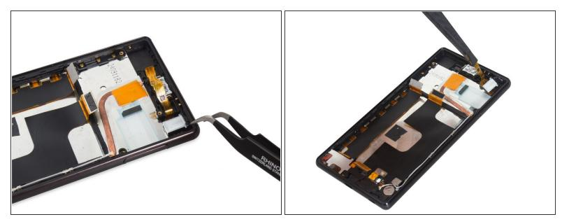
• Cut the adhesive on the top of the audio jack and remove the audio jack assembly.
