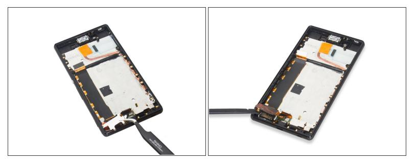
• Remove loudspeaker securing bracket.
