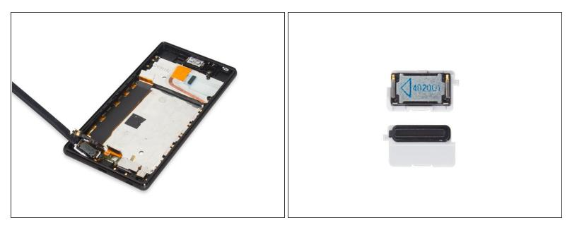
• Remove loudspeaker hidden under the flex.
