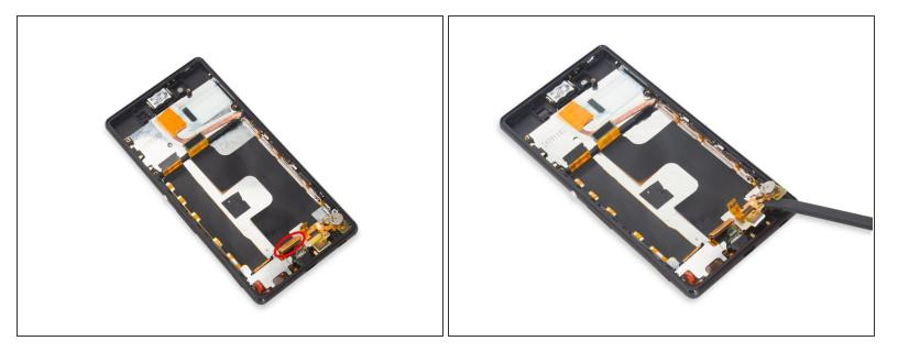
• Release LCD connector there and loosen the bottom of the whole flex.
