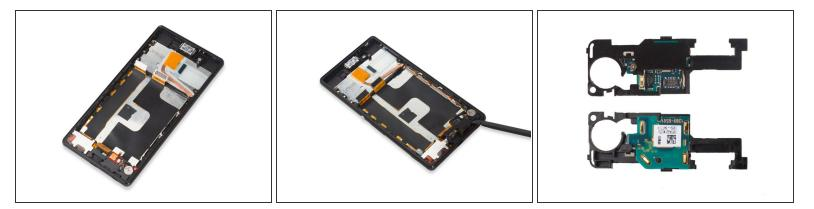
• Release connectors connecting on the antenna logic board and finally remove it.
