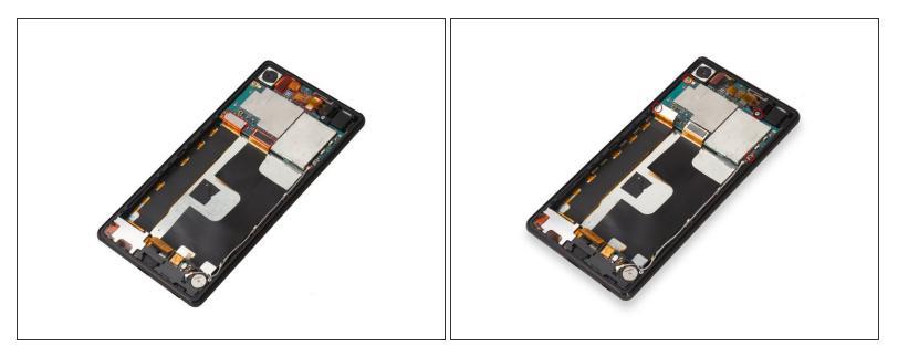
• Release all the connectors on board and remove the screws there.
