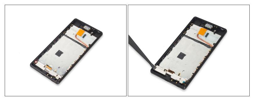
• Remove the metal bracket covering on the screen flex.
