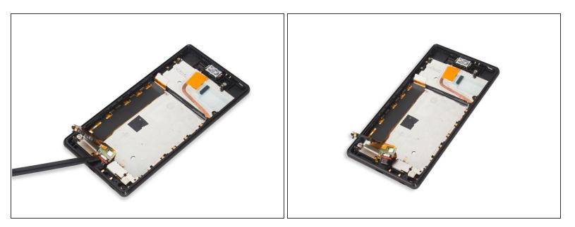
• Push the USB port out of the slot.
