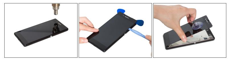
• Remove LCD screen carefully.
