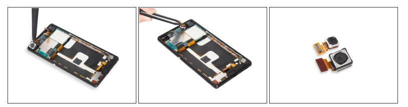
• Remove rear camera and front camera.
