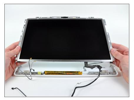
Raise the bottom edge of the LCD assembly slightly, then slide it down slightly to free its upper edge from a
