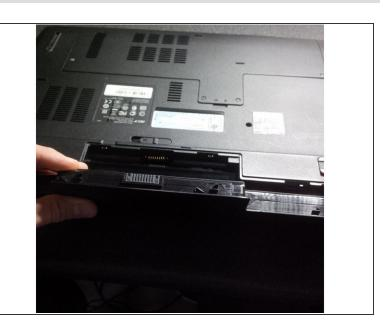
Remove the battery by sliding the locking latch to the right and pull the battery out.
