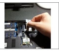
To remove the hard drive, undo the screw that holds it in place and carefully pull the HDD to the right.
