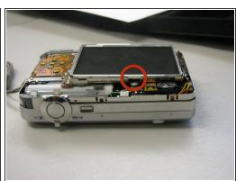
Use the tweezers to pry the LCD screen off from the openings. There are 5 spots that the tweezers can go in to pry the LCD screen off (see attached pictures).
