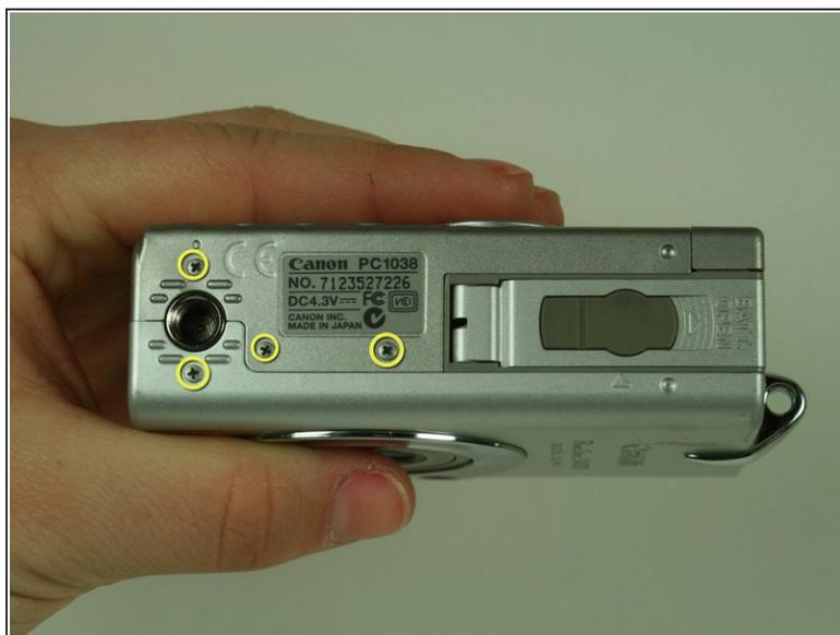
**i** Unless otherwise stated, a #00 philips screwdriver will be used to remove screws.
