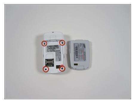
• Remove the 4 (4.7mm) philips head screws.
