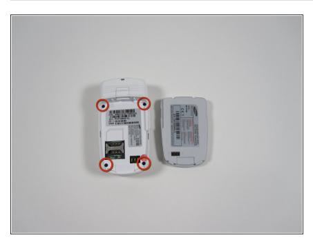
Remove the 4 (4.7mm) philips head screws.
