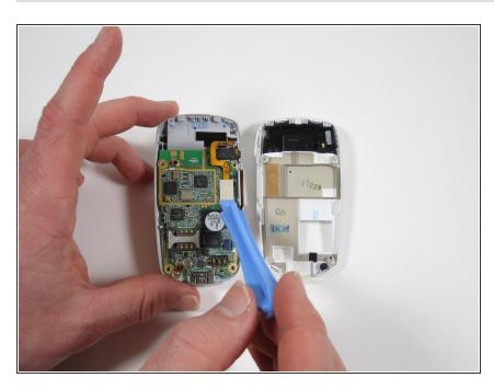
Remove the ribbon wires connecting to the screen using the pry tool.
