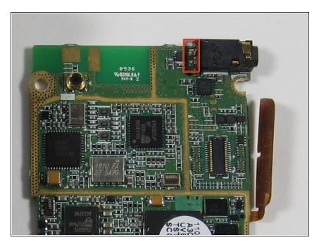
Solder connections can be accessed to replace head phone jack.
