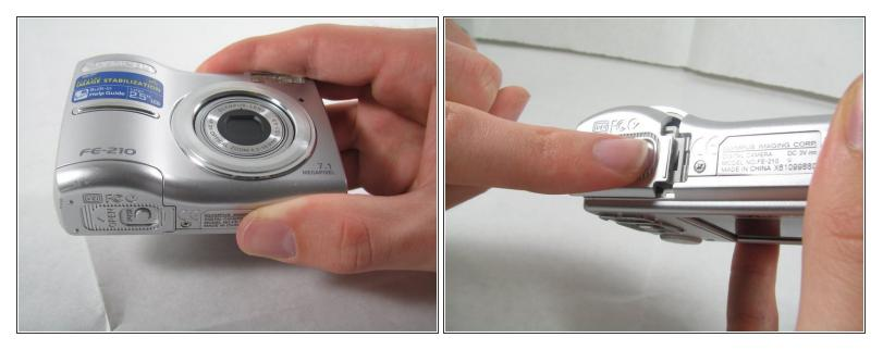
• The battery compartment is located on the bottom side of the camera. Push the button in, and slide the cover to get access to the batteries.
