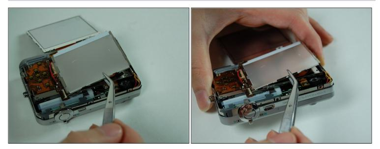
• Using a pair of tweezers, pry off the LCD casing.
