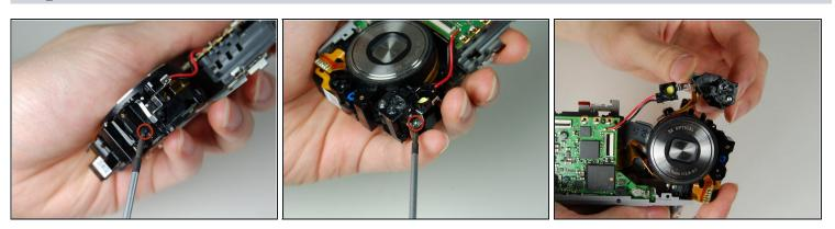
• On the front side of the indicator lamp remove the screw using the Phillips #00 screwdriver.
