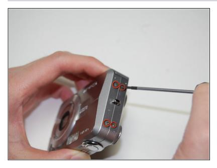
• Using the Phillips #00 screwdriver, remove the four screws from the side opposite of the speaker.
