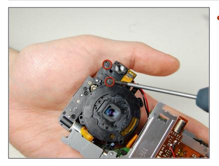
• On the backside of the camera where the indicator lamp is located, remove the two screws using the Phillips #00 screwdriver.
