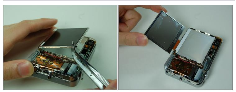
• Lift the LCD screen and move it to the other side.
