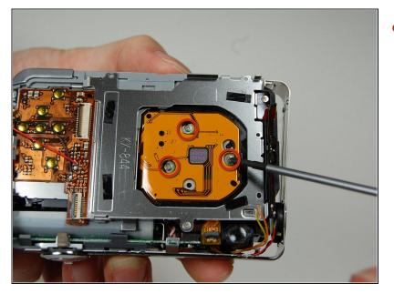
On the back of the camera where the LCD screen was, remove the 3 screws located behind the lens using the Phillips #00 screwdriver.
