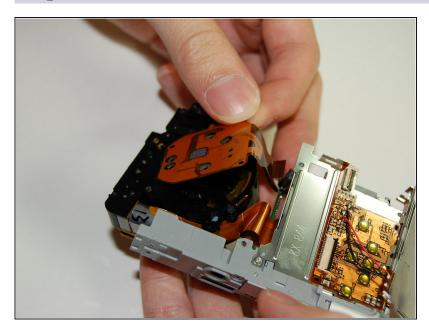
• Remove the large orange ribbon previously held in by screws from the camera.
