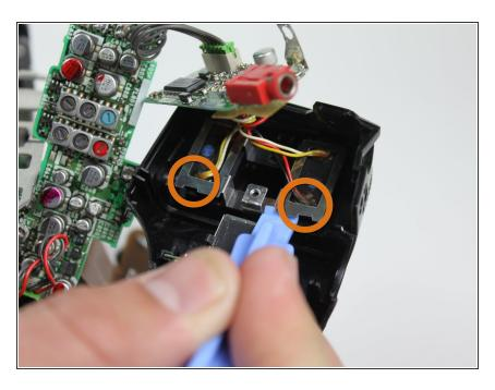
Pull up metal brackets with plastic removal tool.
