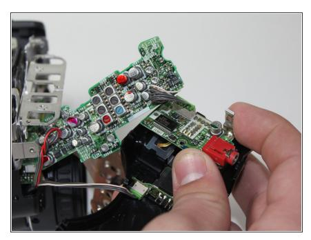
Pull the circuit board up and away from the microphone case.
