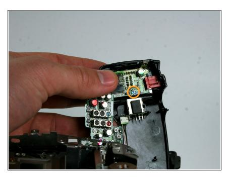
Unscrew the blue screw behind microphone and remove it from the video camera 1x3.6mm.
