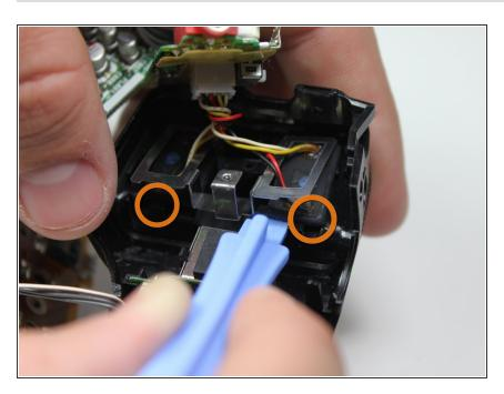
With the plastic removal tool, pry up the microphone housing units. This will allow access to the camcorder microphone.
