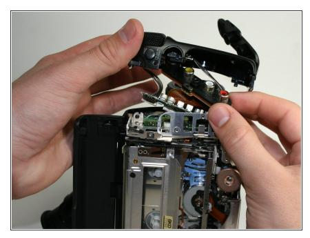
Pull the audio/video inputs underneath the microphone assembly. The inputs should still be connected to the circuit board.
