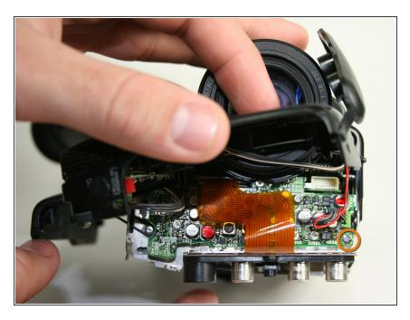
Remove the single 3.6 mm screw at the front of the video camera on the circuit board.
