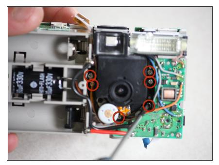
Use the Phillips #00 screwdriver to remove the six screws that secure the camera lens.
