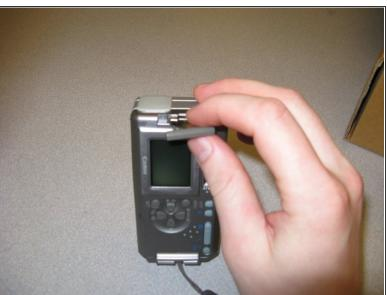
Remove the screen battery located to the left of the screen.
