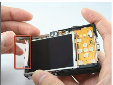
Use the spudger to remove the L-shaped bar from the left-side of the LCD screen.
